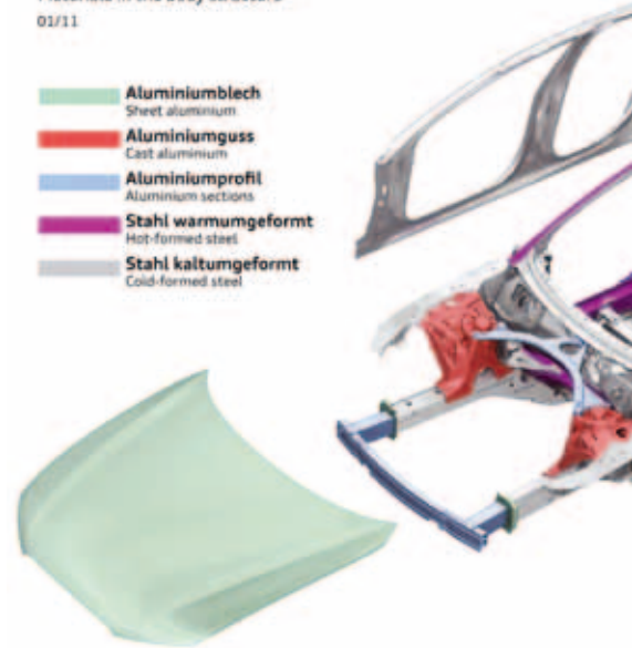
Karosseriematerialien Materials in the body structure 02/11
