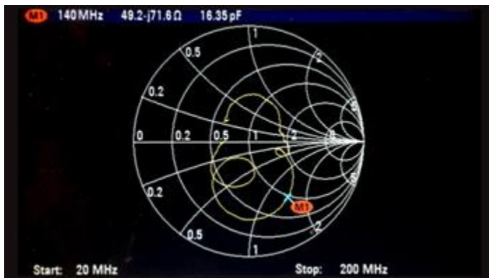
Figure 19 Measured S_{11} of an antenna for a VHF/UHF radio, from 20 to 200 MHz.
