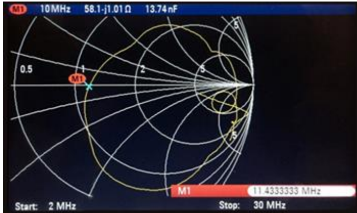
Figure 3 Measured impedance of a 2 x 5 m non-resonant dipole antenna from 2 to 30 MHz.
