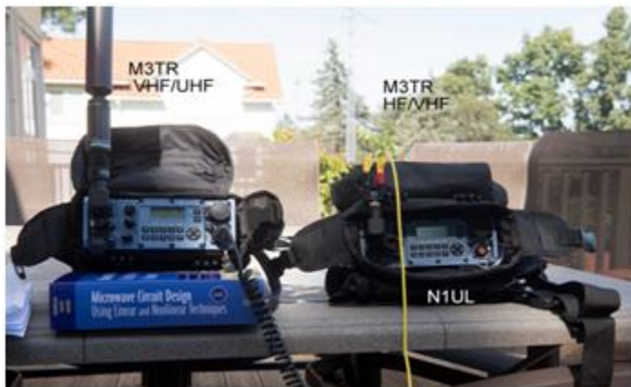
Figure 20 VHF/UHF (left) and HF/VHF (right) manpacks. The UHF/VHF manpack shown uses a thick vertical pole antenna, and the HF manpack uses a 5 m dipole (the yellow wire).
