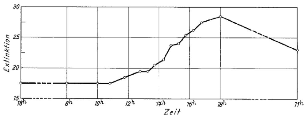
Fig. 1. Photometric measurement of turbidity in growing "Findlay" culture
